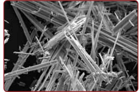
▲ MICROSCOPY IMAGE OF ASBESTOS FIBERS
