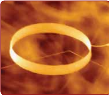
▲ ZINC OXIDE NANOSTRUCTURE synthesized by a vapor-solid process. (Image courtesy of Prof. Zhong Lin Wang, Georgia Tech)
