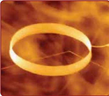
▲ ZINC OXIDE NANOSTRUCTURE synthesized by a vapor-solid process.
